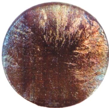
**Fig. 3** OCMG-processed Gd-Ba-Cu-O Bulk (Single-domain 48 mm  $\phi$  sample)
