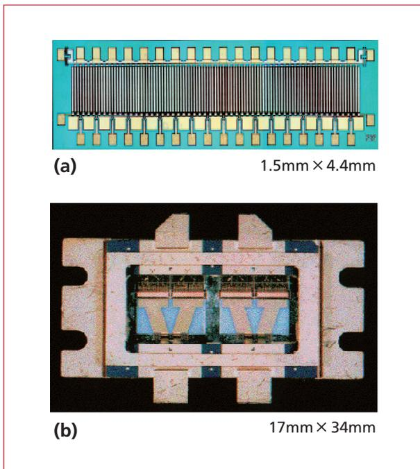
**Fig. 9:** Heterojunction FETs with field plates. (a) Photograph of a chip with a multi-cell structure consisting of a heterojunction FET chip with field plates (chip dimensions: 1.5 mm  $\times$  4.4 mm). (b) Surface photograph of an amplifier with a partial matching circuit that incorporates four FET chips in the same package.
