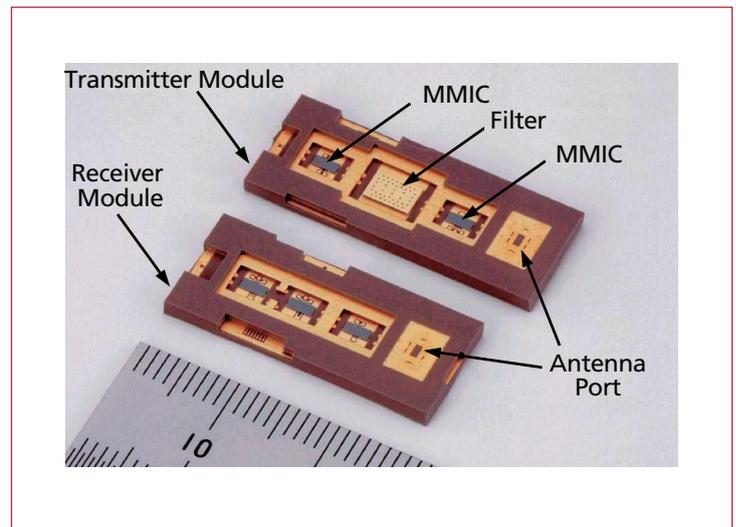
**Fig.10:** Photograph of miniature 60 GHz band transceiver modules. The transmitter module incorporates three types of MMIC—a frequency multiplier, a modulator and a transmitter amplifier. The receiver module incorporates two types of MMIC—a low-noise amplifier and a demodulator—and a bandpass planar filter.
