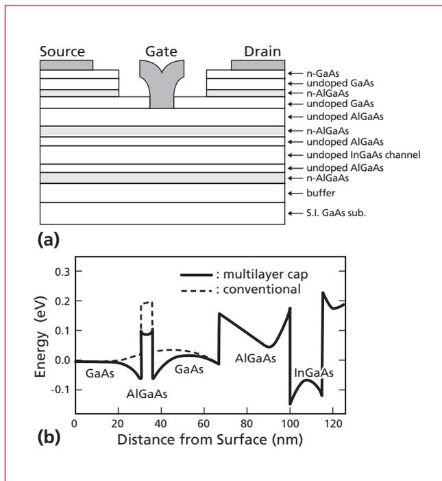
**Fig. 2:** A heterojunction FET with a multilayer cap structure. (a) Cross-sectional structure. (b) Conduction band energy distribution under the ohmic electrode. The use of a multilayer cap structure reduces the potential barrier at the n-AlGaAs layer near the surface.
