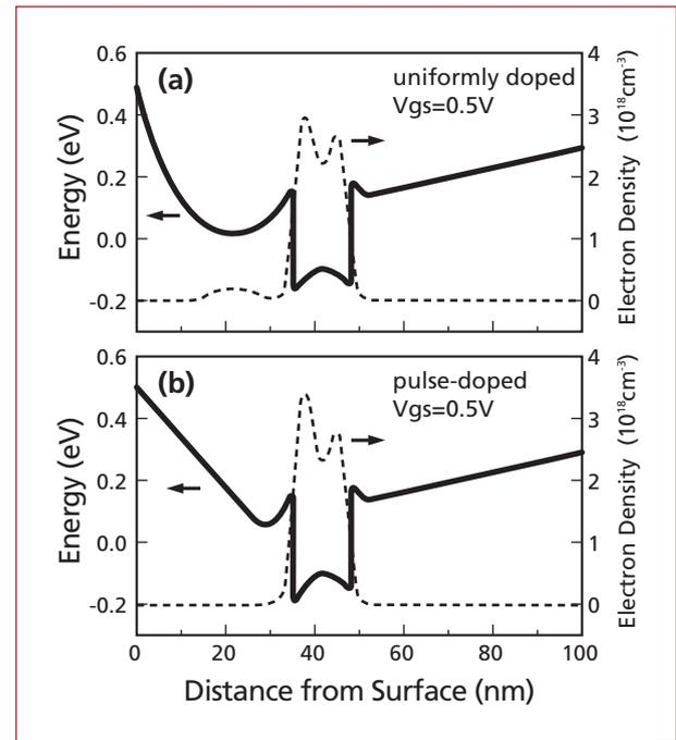
Fig. 1: The distribution of conduction band energy and electron concentration across double-doped/double heterojunctions. (a) Uniformly doped structure. (b) Pulse-doped structure. In the uniformly doped structure, it can be seen that electrons spread out into the AlGaAs electron supply layer.
