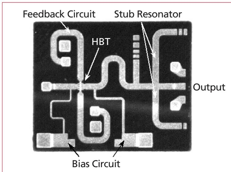
Fig. 11: A 38 GHz MMIC oscillator. An HBT with a graded composition InGaAs base structure is used as the active element. When detuned by 1 MHz, this oscillator has a favorable phase noise of  $-114$  dBc/Hz.
