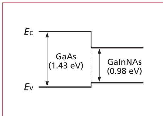
Fig. 6: Relationship between the band positions in GaAs and GalnNAs. Most of the difference in bandgap energy appears as an energy discontinuity at the conduction band side.
