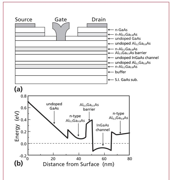
**Fig. 3:** A heterojunction FET with an  $\text{Al}_{0.5}\text{Ga}_{0.5}\text{As}$  barrier layer. (a) Cross-sectional structure. (b) Conduction band energy distribution under the gate electrode. The introduction of a barrier layer suppresses the injection of electrons from the channel towards the gate electrode.
