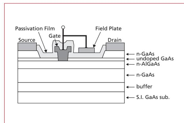
Fig. 8: Cross-sectional structure of a new type of heterojunction FET incorporating a field plate. The field plate is connected to the same potential as the gate electrode.
