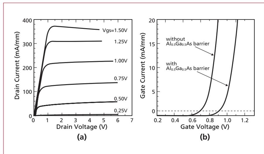
Fig. 4: (a) Drain current vs. voltage characteristics and (b) gate forward characteristics of an enhancement-type heterojunction FET with an  $\text{Al}_{0.5}\text{Ga}_{0.5}\text{As}$  barrier layer. The introduction of a barrier layer improves the forward on voltage by about 0.2 V.
