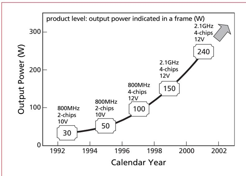
Fig. 7: The year-on-year growth in the performance of high output GaAs FETs developed for mobile phone base stations.
