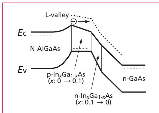
Fig. 5: Energy band diagram of a drift base HBT incorporating a layer of  $\text{In}_x\text{Ga}_{1-x}\text{As}$  with a ramped composition.
