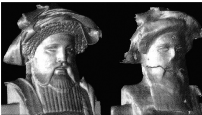
Fig. 1: A bust imaged by X-ray tomography CT
