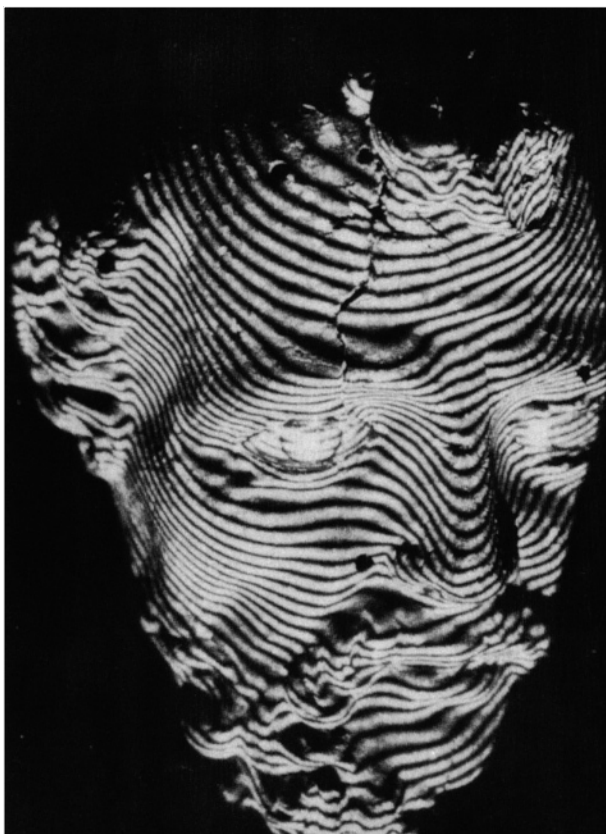
Fig. 3: Interference pattern over a head statue obtained by the holographic interference method
