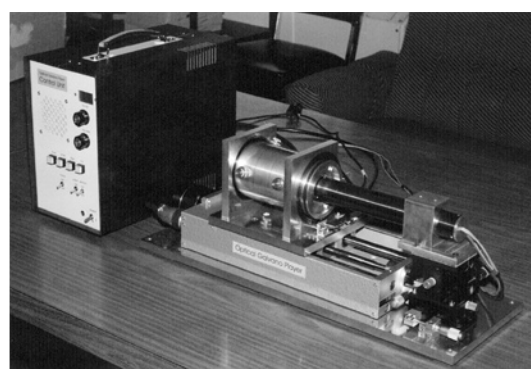
Fig. 9: A reproduction machine for negative cylinders
