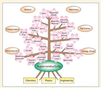
Fig.1 Application Tree of Superconductivity
