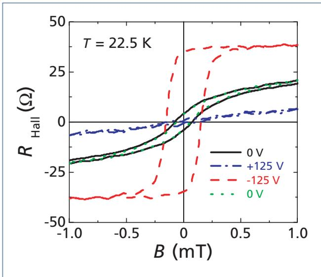
Fig. 7 Gate voltage dependence of Hall resistance in an (In,Mn)As FET structure close to the ferromagnetic transition temperature. When a gate voltage of  $V_G = -125$  V is applied, hysteresis is clearly observed. On the other hand, when  $V_G = +125$  V, the hysteresis disappears. This demonstrates that the applied field is able to switch the device between ferromagnetic and paramagnetic states.<sup>98</sup>
