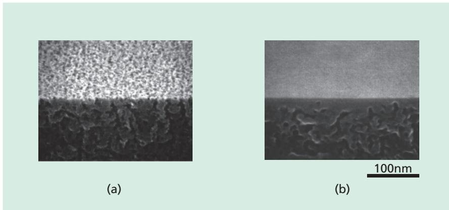
Fig.5 Porous Si surface (a) before and (b) after H<sub>2</sub> pre-baking.
