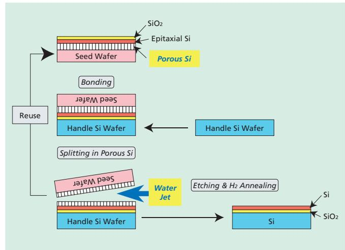
Fig.3 ELTRAN® process flow based on seed wafer reuse.
