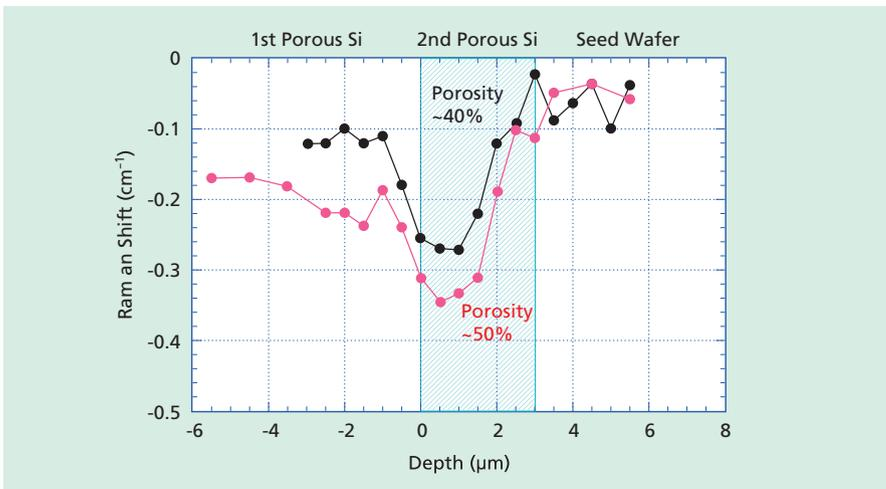
Fig.8 Raman shift depth profile around the 2nd porous Si with different porosity of 40% and 50% just before splitting.
