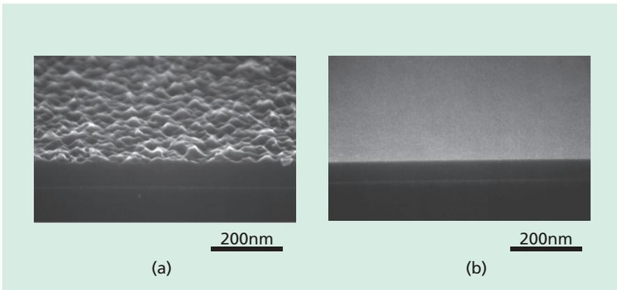
Fig.7 High-resolution, oblique-view micrographs of (a) as-etched ELTRAN® wafers and (b) H2-annealed ELTRAN® wafers.
