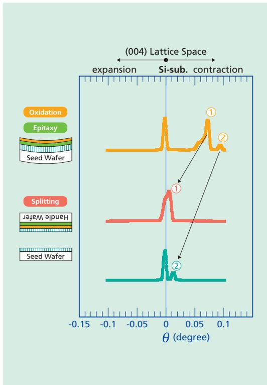
Fig.10 X-ray diffraction rocking curves of each wafer type before and after splitting processes.
