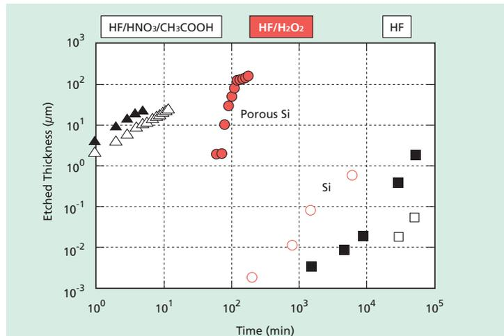
Fig.6 Etching characteristics of porous Si (closed symbols) and nonporous Si (open symbols) obtained through immersion in HF/HNO<sub>3</sub>/CH<sub>3</sub>COOH (triangles), HF/H<sub>2</sub>O<sub>2</sub> (circles) and HF (rectangles) as a function of etching period.
