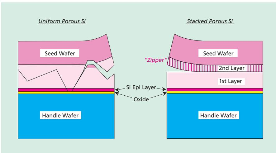
Fig.9 Schematic drawings of crack propagation in double- and single-layered porous Si.
