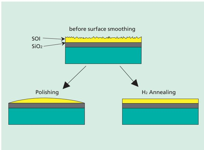
Fig.2 Surface smoothing of SOI wafers by polishing and H<sub>2</sub> annealing.
