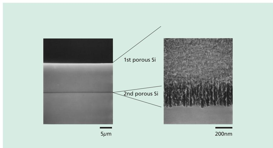
Fig.4 Cross-sectional micrographs of double-layered porous Si formed by changing anodic current.
