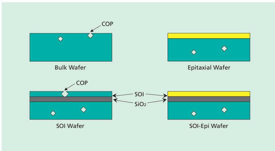
Fig.1 COPs in bulk wafer, epitaxial wafer, SOI wafer and SOI-Epi wafer.
