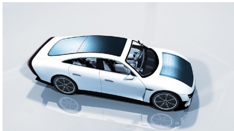
Figure 3 Image of a Cu 2 O/Si tandem solar cell installed in an EV (courtesy of Toshiba)
