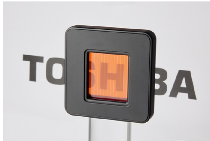
Figure 2 Prototype of 40 mm square transparent Cu 2 O solar cell (courtesy of Toshiba)
